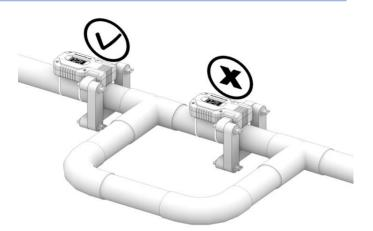
If there is an "electrical circuit", there is a metallic connection in front of and behind the unit. The voltage breaks down (short circuit).
