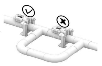
If there is an "electrical circuit", there is a metallic connection in front of and behind the device. behind the device. The voltage breaks down (short circuit).
